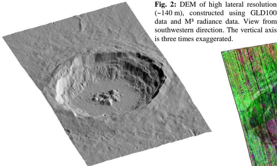
**Fig. 2:** DEM of high lateral resolution (~140 m), constructed using GLD100 data and M<sup>3</sup> radiance data. View from southwestern direction. The vertical axis is three times exaggerated.
