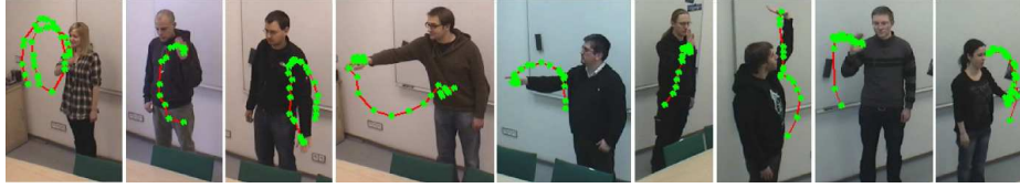
Fig. 1. Examples of the gesture classes (from left to right) “circle”, “come here”, “down”, “go away”, “point”, “stop”, “up”, “horizontal wave”, and “vertical wave”. The extracted 3D trajectories have been reprojected into the image (from [15])
